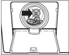
■ Return the lint trap and tighten into place.
